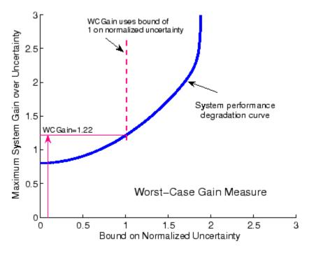
On the graph, this is the vertical coordinate of the performance degradation curve as it crosses the vertical line drawn at the uncertainty bound = 1.
